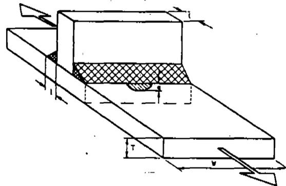
Fig.5: Transverse non-load-carrying stiffener weld.
