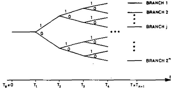
Fig.1: Illustration of event tree with repair of all detected cracks. 0 denotes no repair, while 1 denotes repair.
