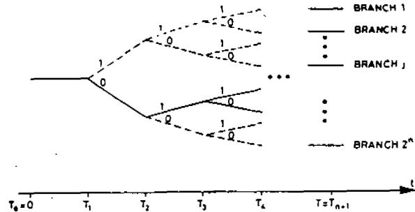
Fig.4: Illustration of event tree with repair of all detected cracks and two inspection results available. 0 denotes no repair, while 1 denotes repair.
