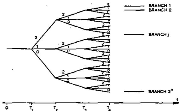
Fig.2: Illustration of event tree with no repair of small detected cracks and weld repair of large detected cracks. 0 denotes no crack detection, 1 denotes no repair of a detected crack, and 2 denotes weld repair.
