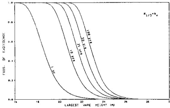
Fig.8 Probability of exceedance of the largest value of wave height
