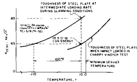
Fig. 3 Example of Toughness Behavior of Steel Plate Exhibiting 13.5 ft-lb at  $-10^\circ\text{F}$ .
