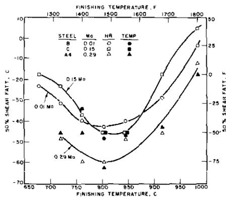
Fig. 5 Effect of Finishing Temperature and Molybdenum Content on the CVN 50% Shear FATT of Hot-Rolled and of Tempered Plates of Low-Carbon Mn-Mo-Cb Line-Pipe Steels (Reference 19).
