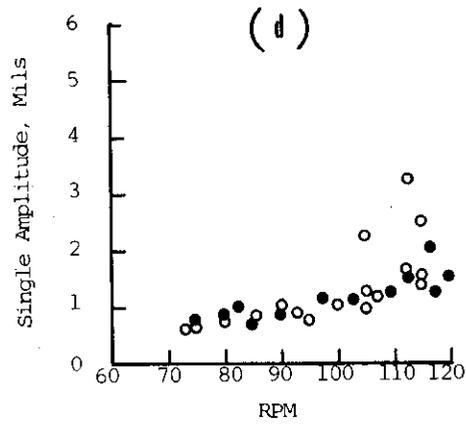
Longitudinal Vibration of Forward End of Bull Gear Shaft
