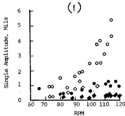
Longitudinal Vibration of High Pressure Turbine
