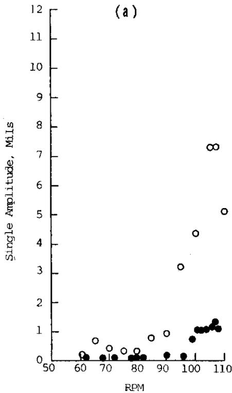
Vertical Vibration of Elevator Casing at Upper Deck
