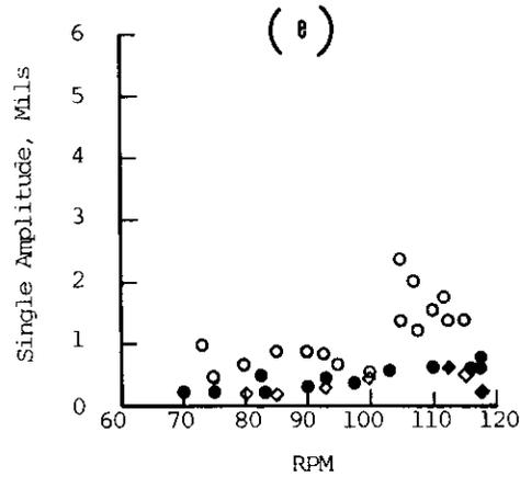
Longitudinal Vibration of Gear Case
