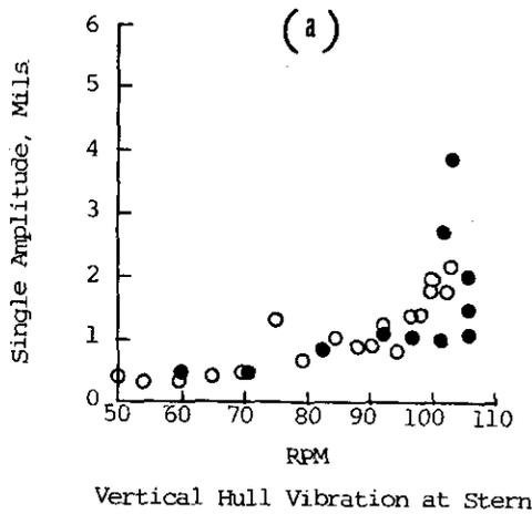
Vertical Hull Vibration at Stern
