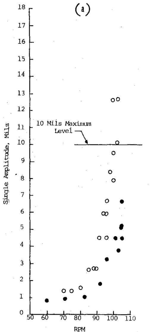
Longitudinal Vibration of Thrust Bearing
