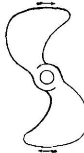
Figure A3 - Hirsch's Screw Propeller
