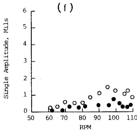
Longitudinal Vibration of Gear Case
