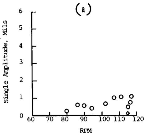
Vertical Vibration of Thrust Bearing
