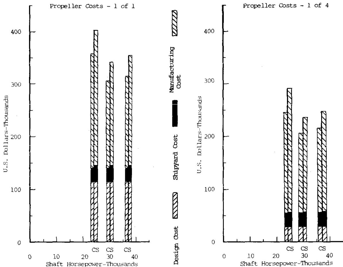
Figure 28 - Cost Factors for Conventional and Highly Skewed Propellers
