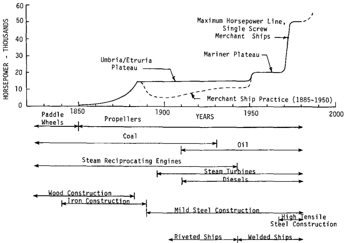
Figure B1 - Growth of Single Screw Merchant Ship Horsepower and Vibration Excitation Response Factors
