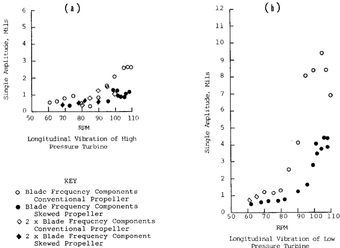
Figure 9 - High Pressure and Low Pressure Turbine Vibration
