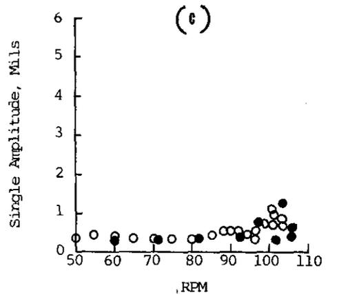
Vertical Vibration of Thrust Bearing
