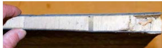
Figure 85. Description of USNA 9 panel that weighs 2.29 lbs/ft<sup>2</sup> (left) and USNA 10 panel at 1.74 lbs/ft<sup>2</sup> (right)
