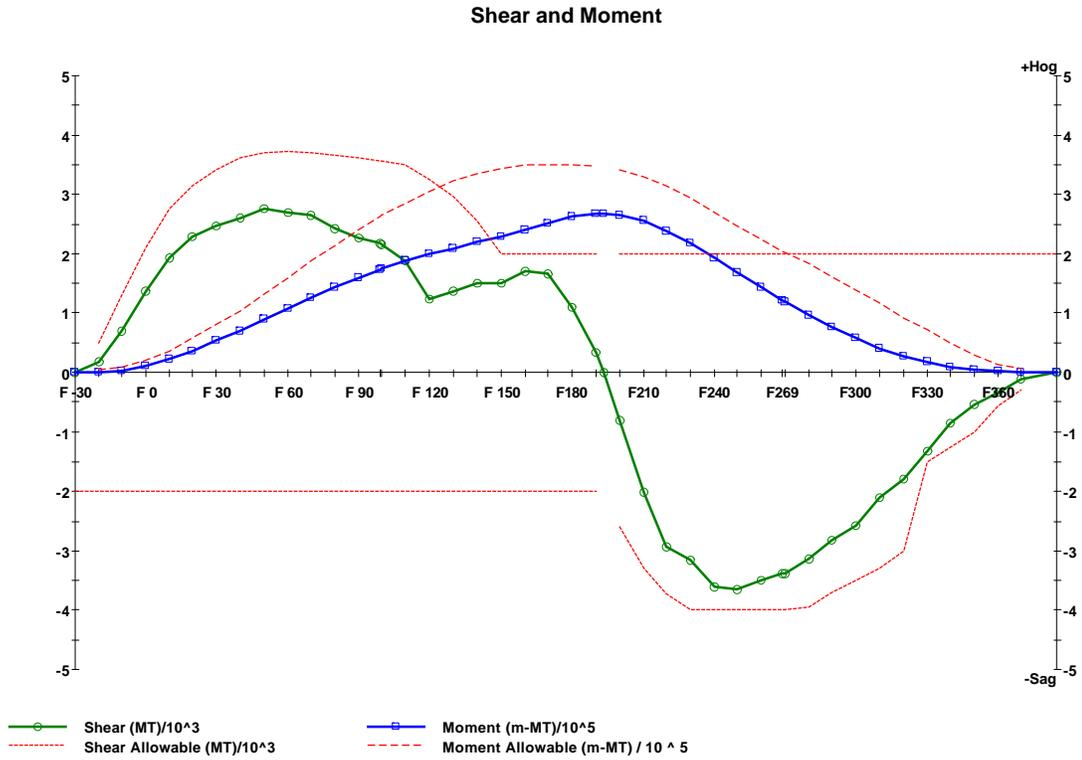
Figure 25 – Minimum hogging moment condition, 2-compartment damage, Hog wave
