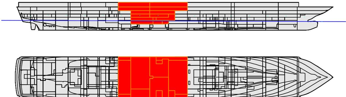
Figure 9 - Flooded compartments for High extent two-compartment damage
