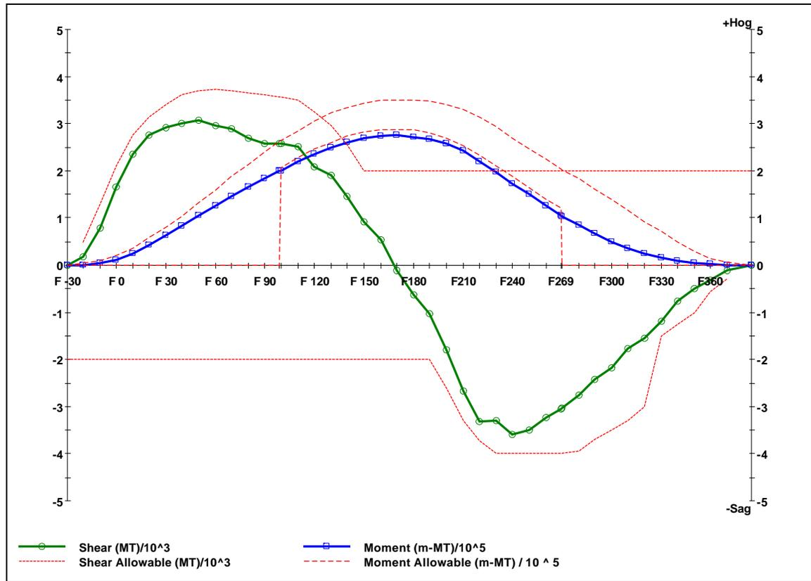
Figure 6 – Still Water Bending Moment (Min. hogging BM intact condition)
