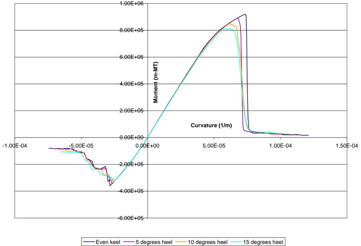
Figure 12 - Ultimate strengths of intact section at different heel angles
