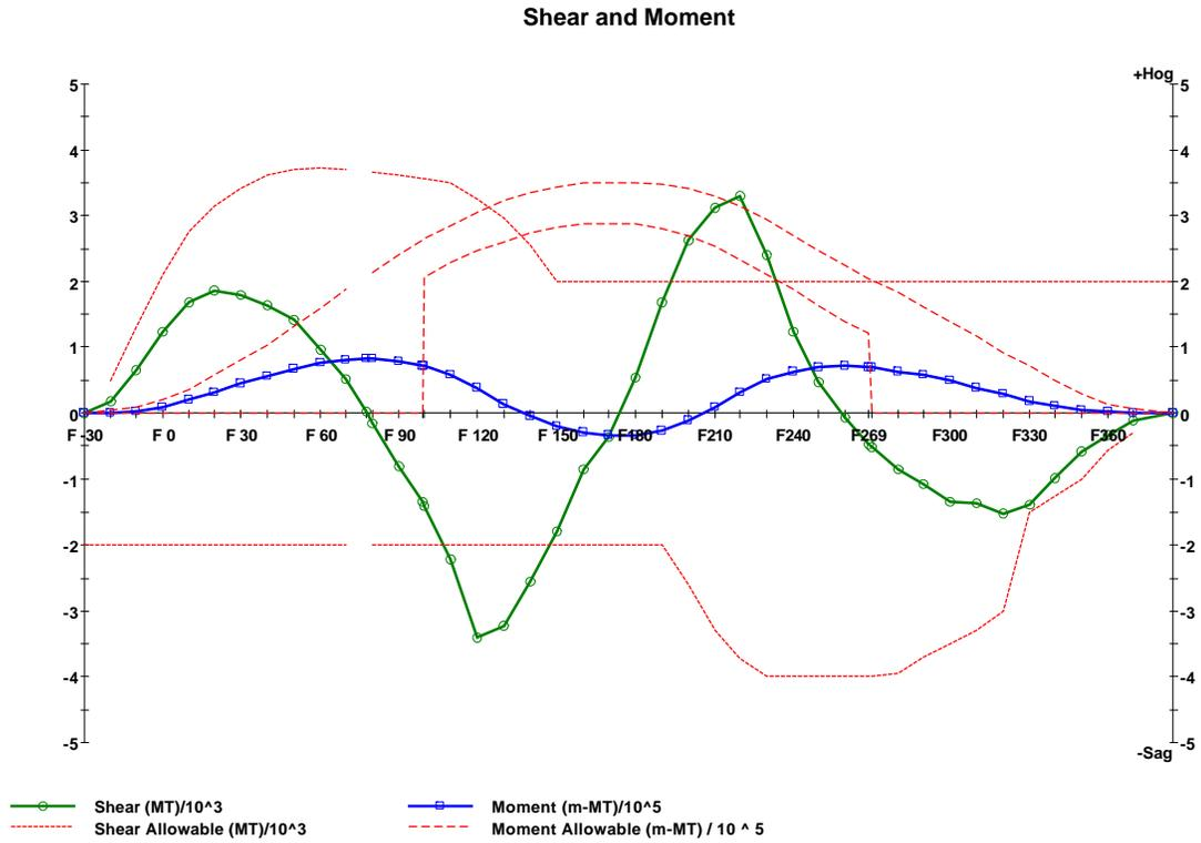
Figure 16 - Minimum Freeboard condition, 4-compartment raking damage, Hog wave
