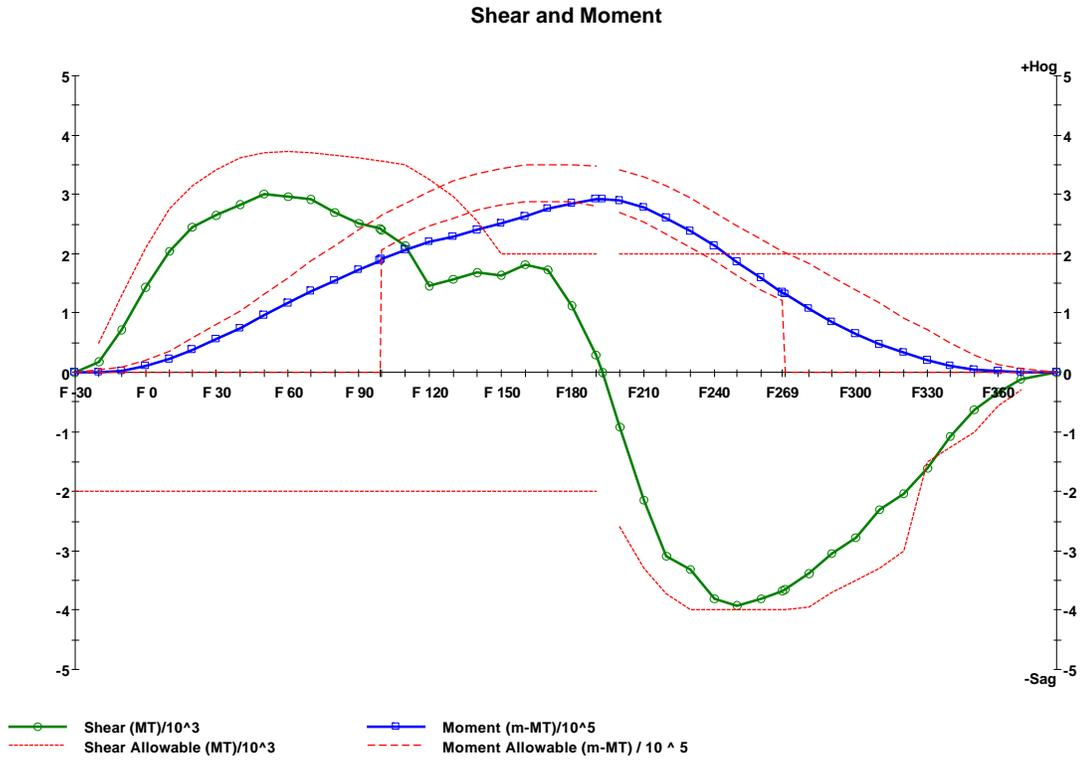
Figure 18 - Minimum Freeboard condition, 2-compartment damage, Hog wave
