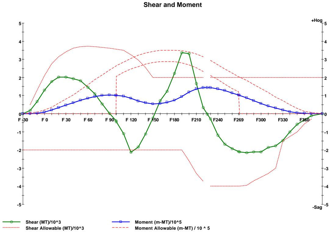
Figure 20 - Minimum Freeboard condition, 3-compartment damage, Hog wave
