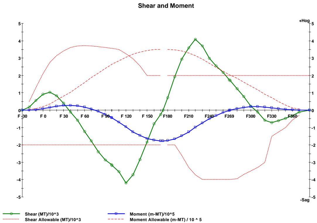
Figure 24 – Minimum hogging moment condition, 4-compartment raking damage, Sag wave
