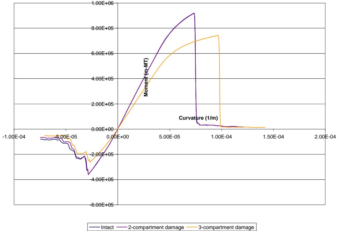
**Figure 14 - Ultimate strengths of damaged structure in upright condition**
