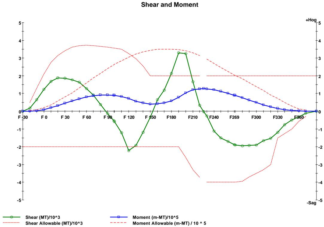
Figure 27 – Minimum hogging moment condition, 3-compartment damage, Hog wave
