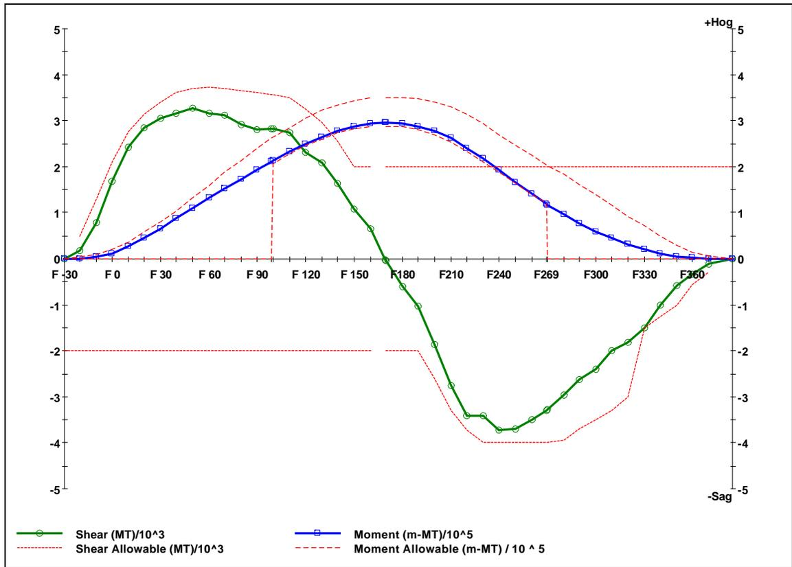
Figure 4 – Still Water Bending Moment (Min. Freeboard intact condition)
