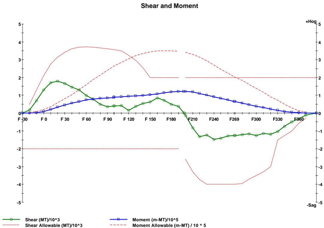
Figure 26 – Minimum hogging moment condition, 2-compartment damage, Sag wave
