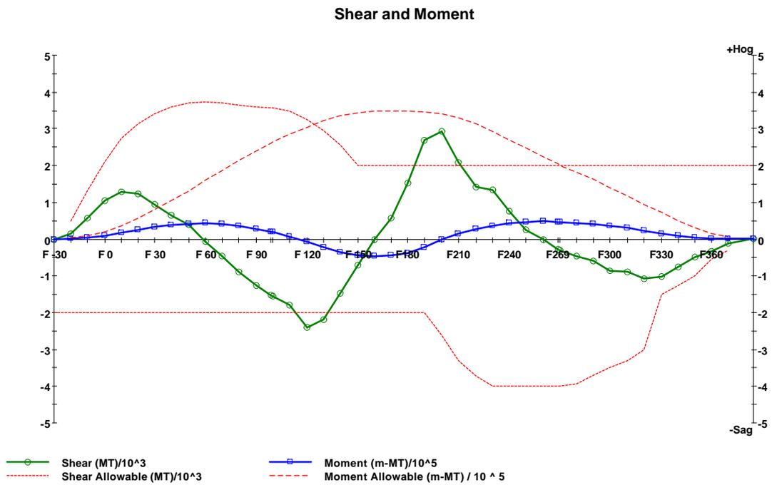
Figure 23 – Typical Departure condition, 3-compartment damage, Sag wave
