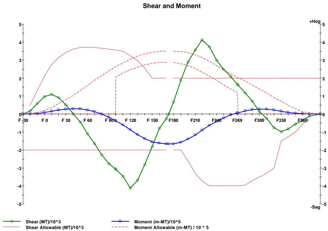
Figure 17 - Minimum Freeboard condition, 4-compartment raking damage, Sag wave
