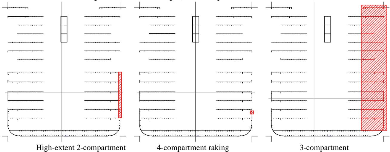
Figure 13 - Damage Extents
