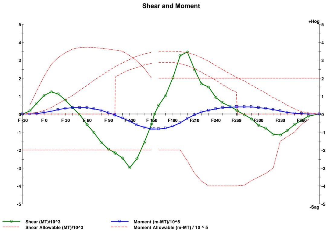
Figure 21 - Minimum Freeboard condition, 3-compartment damage, Sag wave
