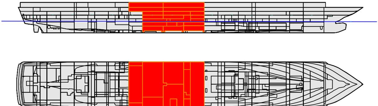
Figure 11 - Flooded compartments for three-compartment damage
