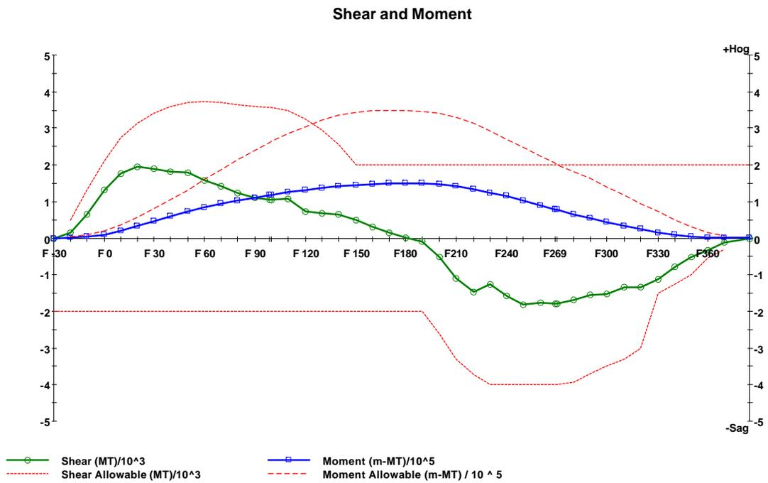
Figure 22 – Typical Departure condition, 2-compartment damage, Sag wave
