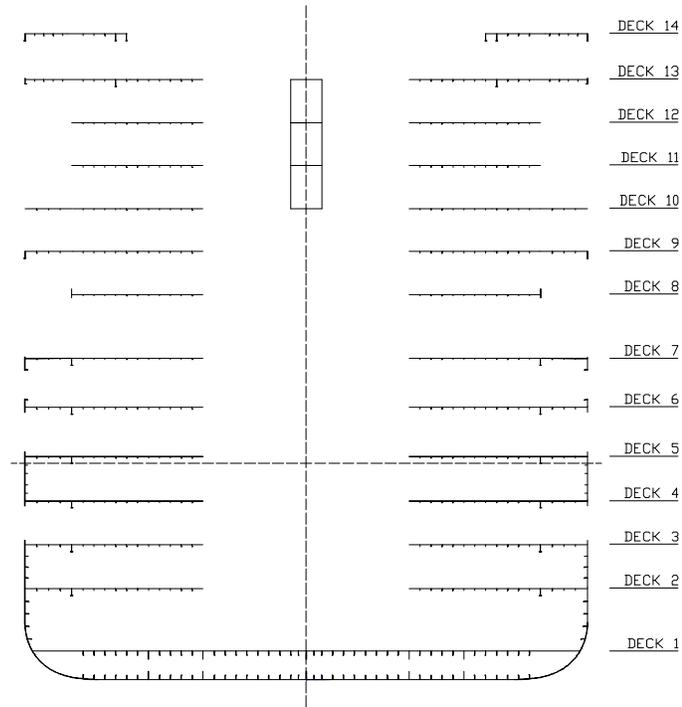
**Figure 3 – “Reduced” Midship Section with openings deducted**
