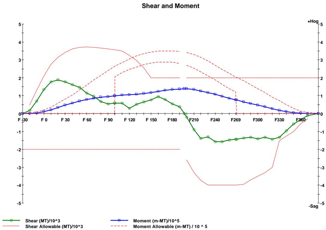
Figure 19 - Minimum Freeboard condition, 2-compartment damage, Sag wave
