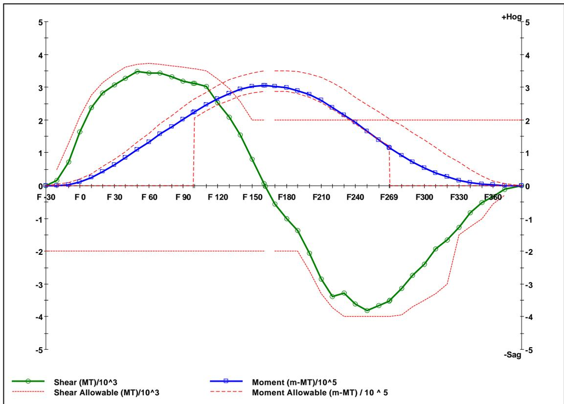
Figure 5 – Still Water Bending Moment (Typical departure intact condition)
