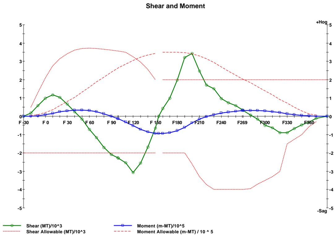
Figure 28 – Minimum hogging moment condition, 3-compartment damage, Sag wave
