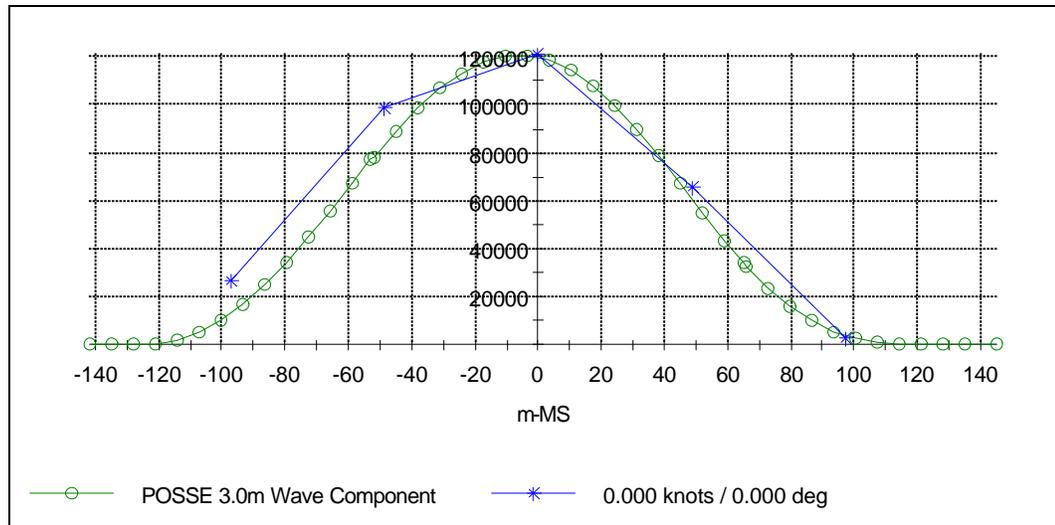
Figure 7 - Dynamic Moment in a 3.5 m Seaway and the Equivalent Static Wave for 24 hours of exposure
