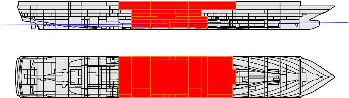
Figure 10 - Flooded compartments for raking four-compartment damage
