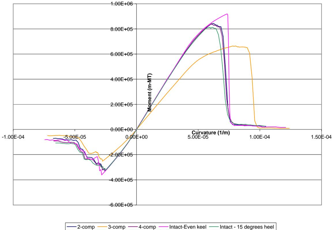
Figure 15 - Ultimate strengths of damaged structure in Max Freeboard Draft Condition
