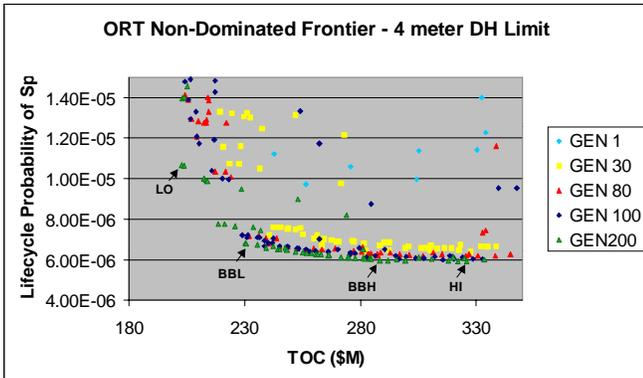
Figure 11 – Spill Probability vs. Cost Frontier
