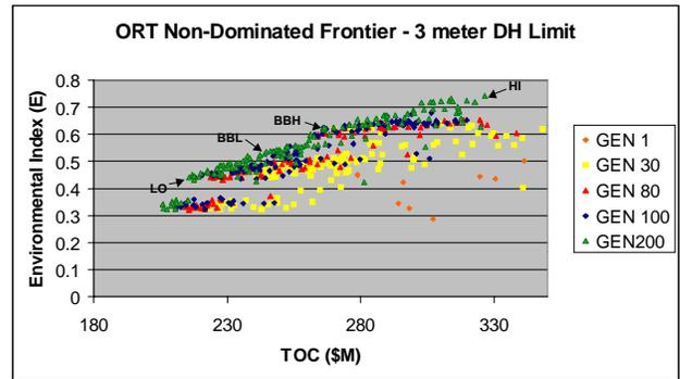
Figure 13 – Environmental Index vs. Cost Frontier (w/3 meter double hull limit)
