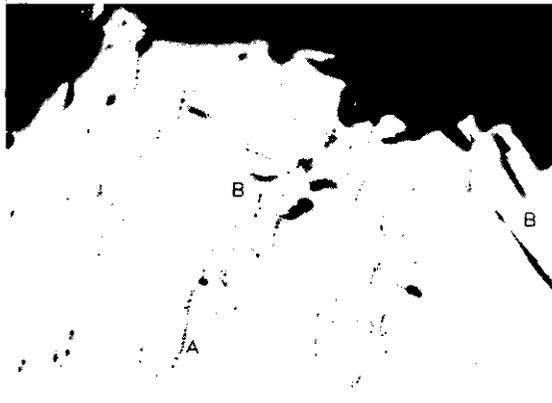
(a). Voids in neck of F4-100 (-90C) 32.3% reduction in area. Note cracked carbides at (A) and cleavage cracks at (B). Fracture about 10% fibrous.
