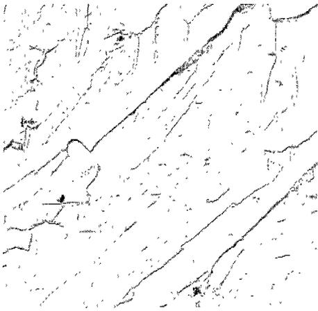
FIG. 21. BRITTLE FRACTURE AT ROOM TEMPERATURE IN UNDEFORMED METAL. NOTE RIVERS AND TONGUES. x 2000
