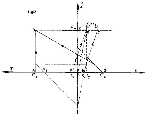
FIG. 12b. On the left side diagram  $\sigma$  versus nominal stress, for unnotched specimen with residual stresses ( $\sigma_t$  and  $\sigma_c$ ).
