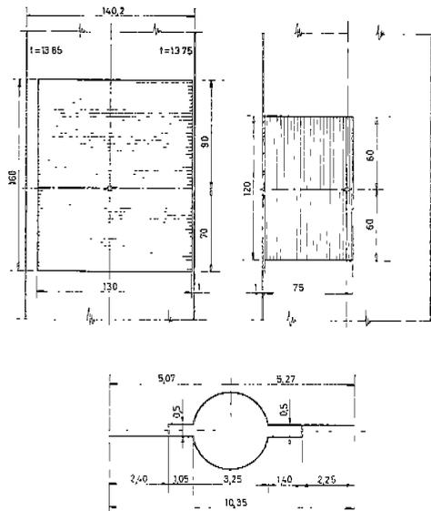
FIG. 3. SPECIMEN WITH SHORT CRACK.
