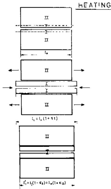
FIG. 34. WELDING OF WIDE OR STIFF SPECIMENS ENTAILS DURING HEATING PLASTIC STRAINING IN COMPRESSION.
