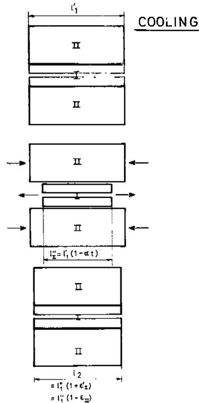
FIG. 35. WELDING OF WIDE OR STIFF SPECIMENS ENTAILS DURING COOLING PLASTIC STRAINING IN TENSION.
