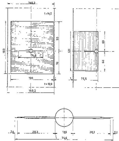
FIG. 4. SPECIMEN WITH LONG CRACK.
