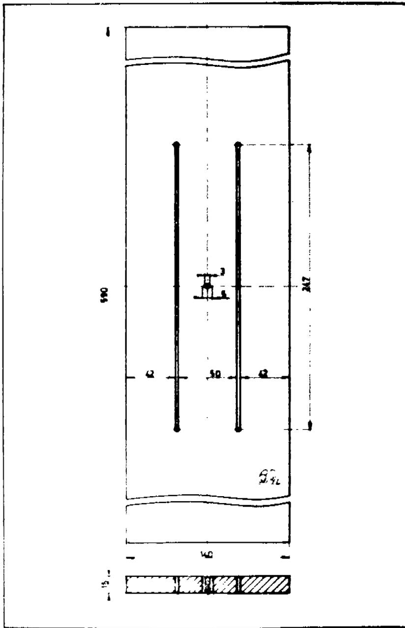
FIG. 36. FRAME-TYPE SPECIMEN USED TO STUDY THE CONDITIONS NECESSARY TO PROVOKE LOW-STRESS BRITTLE FRACTURE.
