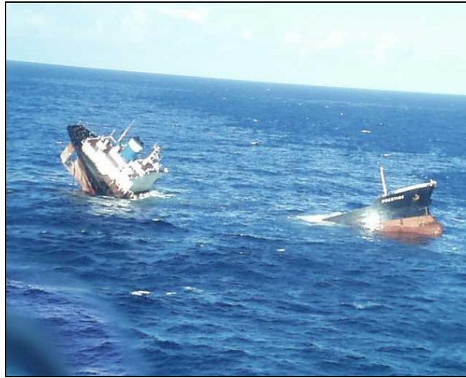
Figure 5. PRESTIGE after hull separation.
