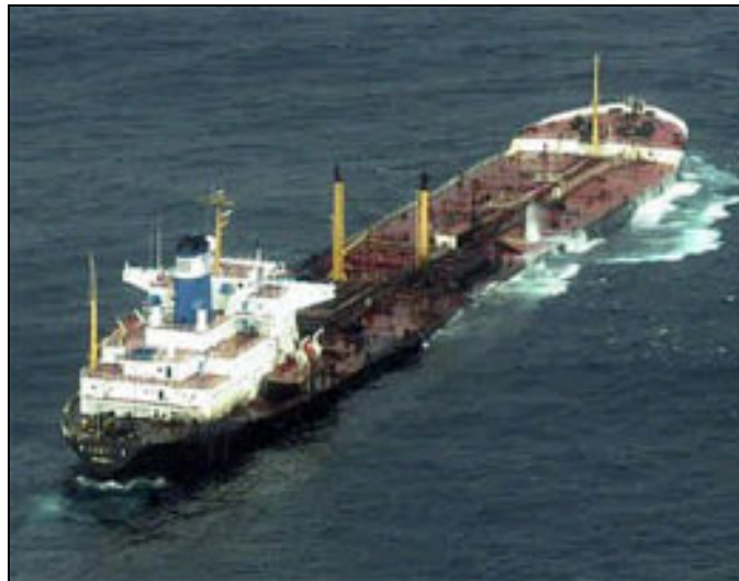
Figure 4. Prestige after counter-ballasting.
